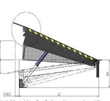
BH = building height O = effective working range above platform L2 = platform length U = effective working range under platform
